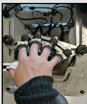
Figure 3: How the hand is placed in the MyHand™ System. Each Finger is placed in separate finger cups and adjusted accordingly
